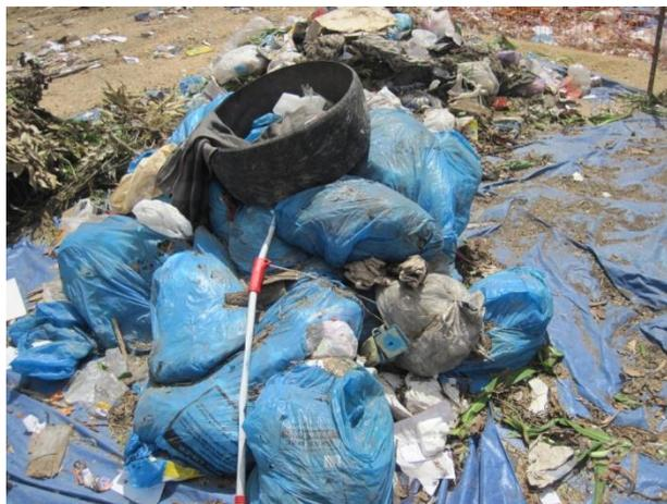
**Figure 3-5 Sample placed on plastic sheet to allow fines to be collected**
