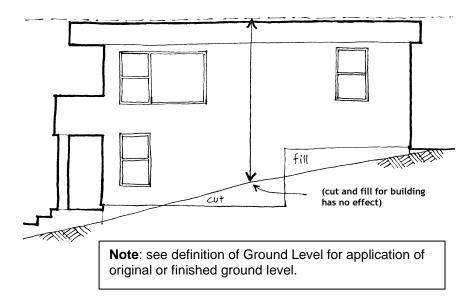
Height is measured from a level which is the average original ground level determined from points around the foundations. Building plans should show in plan view the points used in calculating mean ground level.
