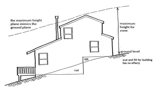
Note: see definition of Ground Level for application of original or finished ground level.
